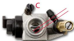
**The idle needle screw is used to adjust the debit of the air. The throttle-valve must be around 0.6 mm in open position. Before you do this, remove first the venturi.**
